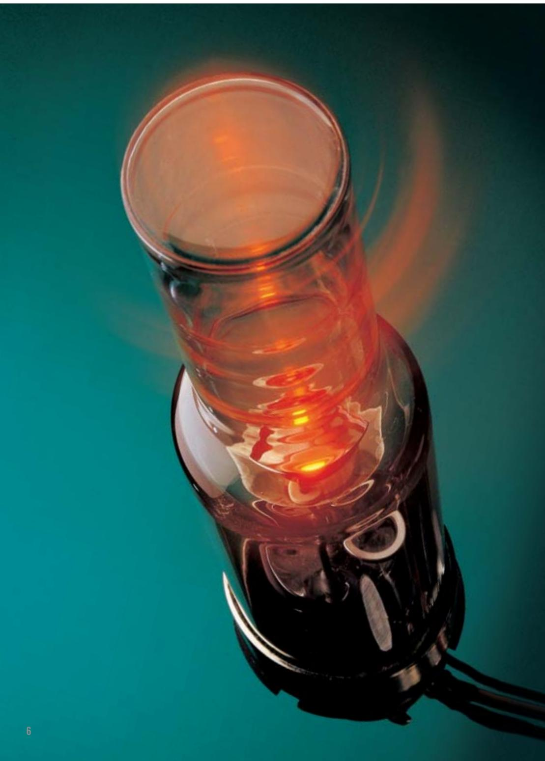
Hollow cathode lamps (HCLs) are a key component for atomic absorption spectroscopy. They consist of a cathode made from the element of interest, an anode and an inert filler gas contained in a glass envelope.
