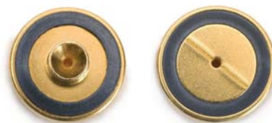
Figure 1 Vespel® rings on both the top and bottom surfaces simplify installation by reducing the torque requirement and eliminating the need for a washer.
